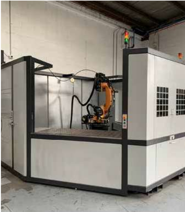
Recently New Touch Industries has been constructing a robot welding unit with an ingenious enclosure to allow continual operations.
